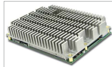
Passive Heat Sink
