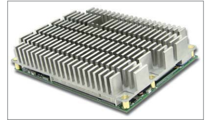
Passive Heat Sink
