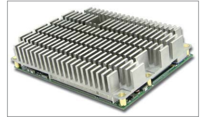
Passive Heat Sink
